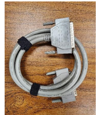
Figure 26 5 ft Wiremapping Cable
