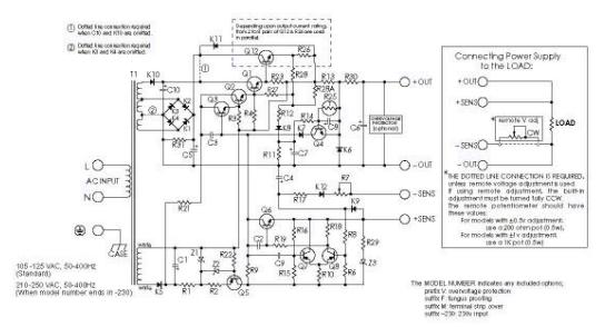
CAUTION: To provide protection from risk of fire, include in the AC input wiring a 250V time-delay fuse with the amp rating listed below: (These fuse ratings are for 115V input models only, contact factory for fuse ratings for 230V input models.)
