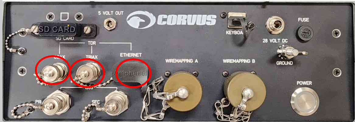
Figure 15 CORVUS Top Panel with Accented TDR Connections
