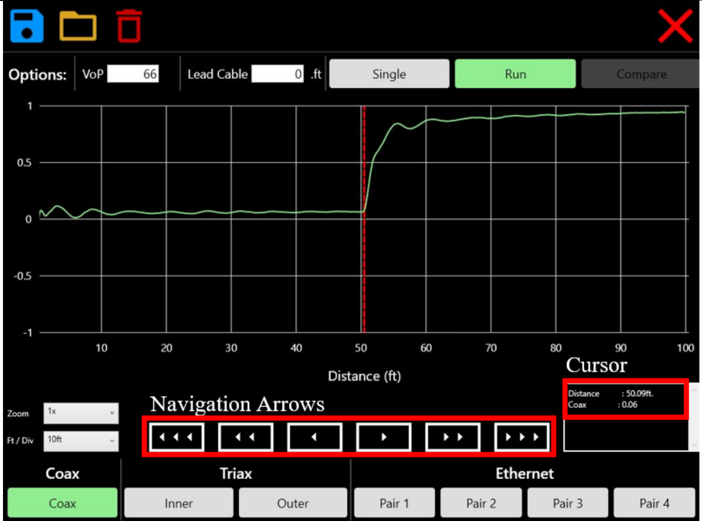
Figure 16 Example 25ft TDR Ethernet Trace
