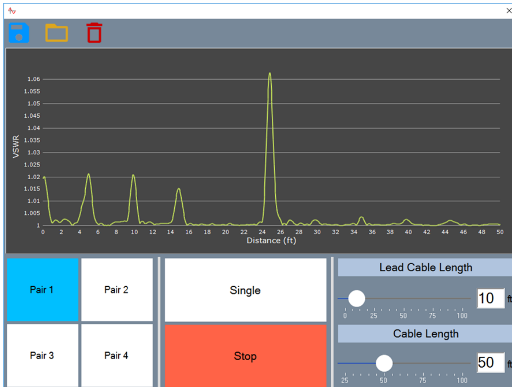
Figure 36 Distance to Fault VNA Display
