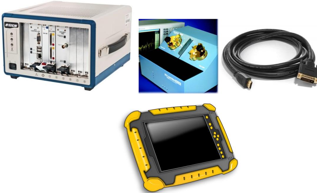
The concept is to integrate a Vector Network Analyzer in VXI format with DragoonITCN's controller and TDR card with Beta LaserMike's balun twisted-pair fixture with a DVI connector adaptor pig-tail and display the GUI DVI cable test result on a Tablet computer. Interfacing the Twisted Pair fixture with the VNA and TDR with operator SW will constitute the basis of this effort, but the overall risk is moderate since the technique of characterizing the DVI cable is understood.
